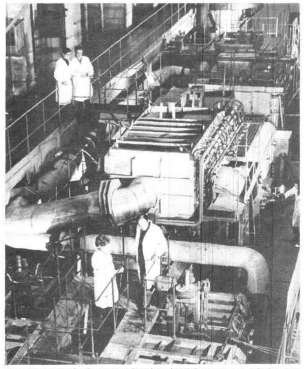
The generator in the Soviet U-02 bench-scale MHD experiment, which used a U.S.-built cryogenic magnet from Argonne National Laboratory in Illinois.
