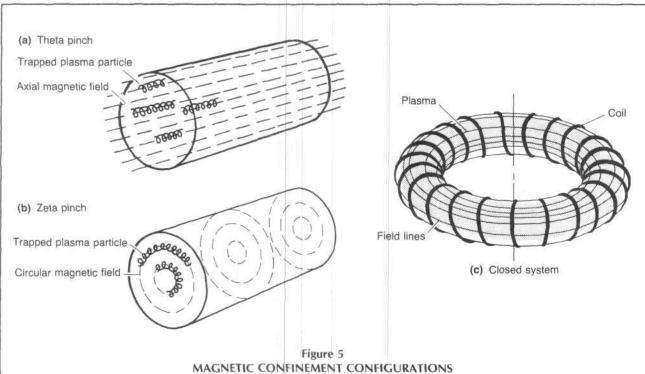
In a, an axial magnetic field traps plasma ions and electrons into spiral orbits along the field lines. A plasma current is induced to flow in a circular fashion, the short way around the cylinder. This generates the magnetic field parallel to the axis of the plasma cylinder. If the induced plasma current is made to increase rapidly, then the intensity of
