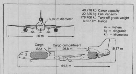
Lockheed's L-1011 TriStar, the cargo airliner the corporation proposes to modify for use of liquid hydrogen  $(LH_2)$  fuel. Inset: Overall dimensions and characteristics of the proposed  $LH_2$  freighter.
